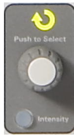
Figure 7 Oscilloscope general-entry control
