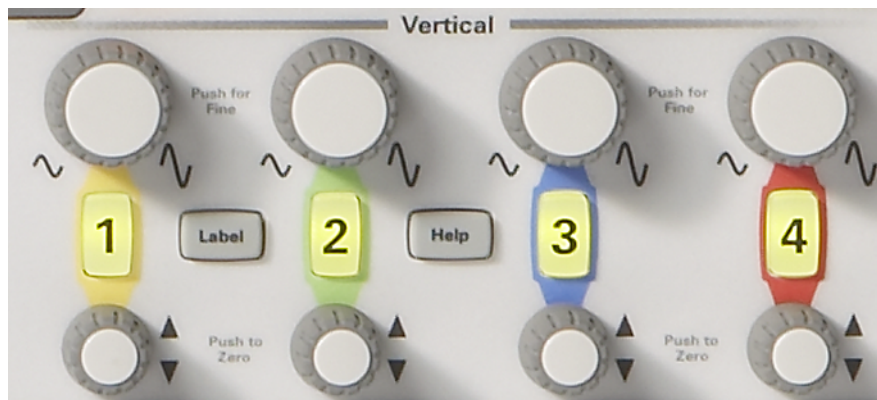
Figure 5 Oscilloscope vertical (Y-axis) controls
