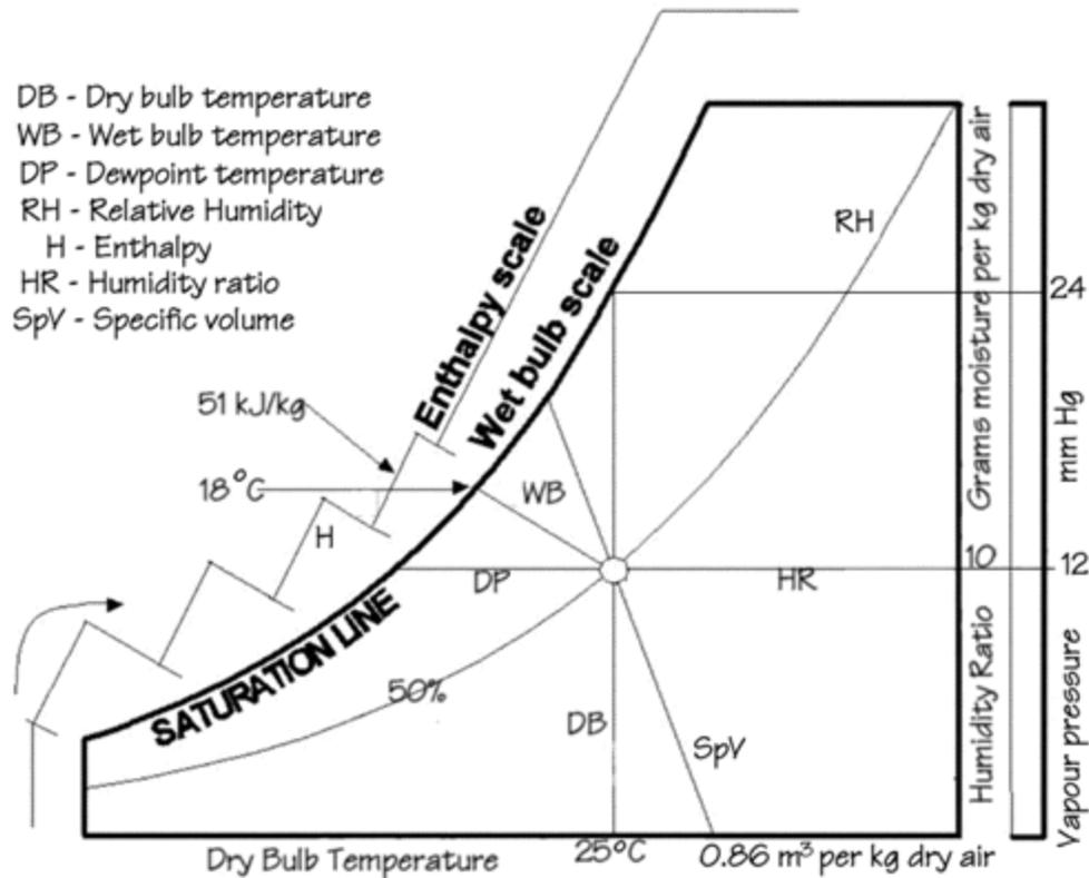
The intersection of the dry bulb temperature line (vertical) and the wet bulb temperature line (diagonal) defines the air:
