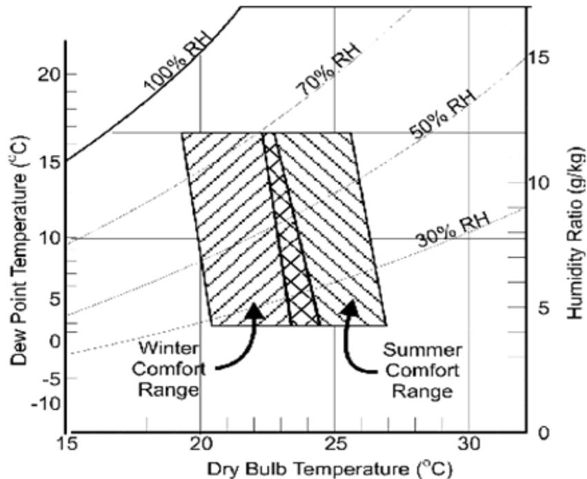
According to the diagram, the highest dry bulb temperature that would be considered “comfortable” in the summer is about 27°C, but to be comfortable, the RH would need to be well below 30%, probably of the order 15%. Similarly, the lowest temperature that would be considered comfortable in the winter is about 19°C, provided that the RH is well above 70%, say about 85%.
