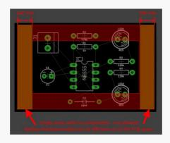
• Every student project will be inspected for design errors. A design rule checking (DRC) process will run for each project to determine if the board meets the constraints set by the PCB machine. If DRC fails, the project will be returned to the student.
